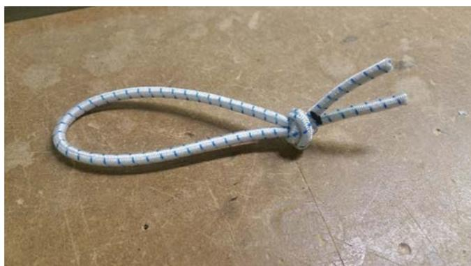
Put the elastic loops where they were originally, close the rescue chute container following the procedure explained in the manual and finally make sure you can extract the rescue chute with ease.
